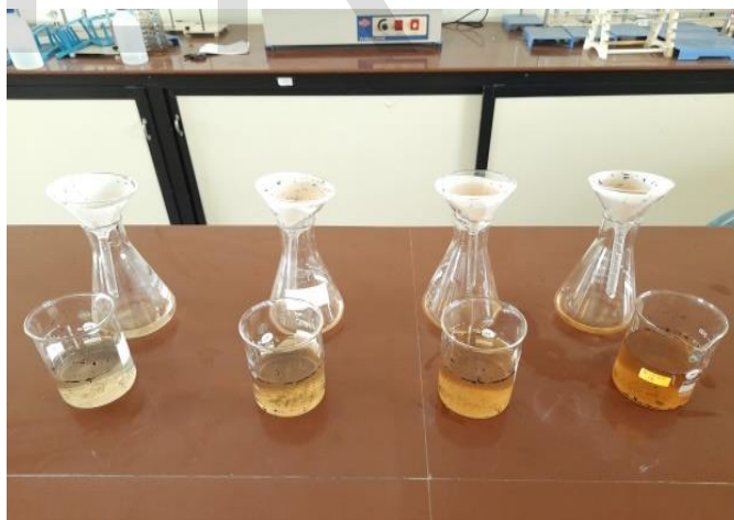
Fig. 3 Filtration of treated synthetic waste water
